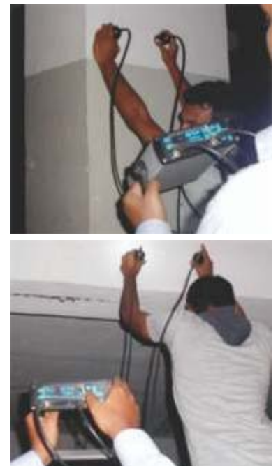
Ultrasonic Pulse Velocity Testing in Column & Beam respectively
