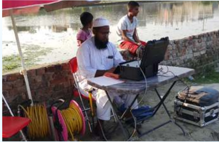
Downhole Seismic Test ASTM D7400
