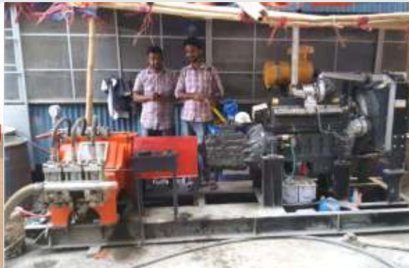
High Pressure Jet Grout Pump System
